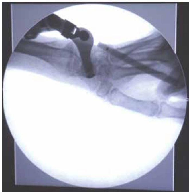
Fig. 13: Wrist module radiotransparency
